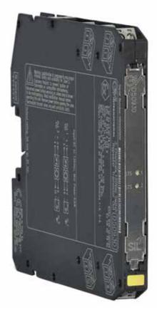
The input switching voltage levels are selected, according to the applied input signal, by means of an internal dip-switch which is overload protected. Mounting of the units can be via standard DIN-Rail or on customized Termination Boards, in Safe Area or in Zone 2, group IIC T4. All models are ATEX, IECEx and SIL certified.
