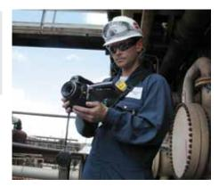
The latest version of the GF320 now embeds GPS data into the image allowing workers to pinpoint the location of the leak or hot spot.
