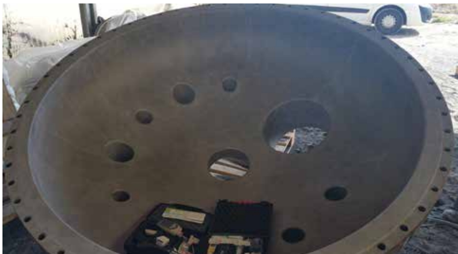
Left: Fig 1. PTFE lining removed Above: Fig 2. Belzona 1593 applied
