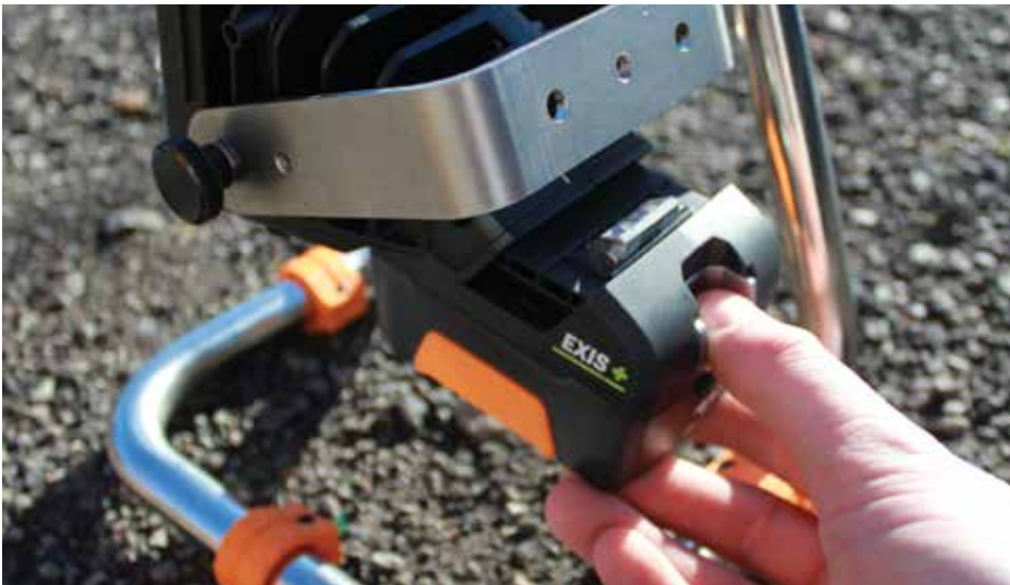
Fig 2.0. A lithium ion I.S. battery pack being hot swapped
