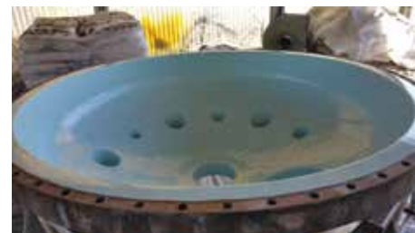
Left: Fig 1. PTFE lining removed Above: Fig 2. Belzona 1593 applied
