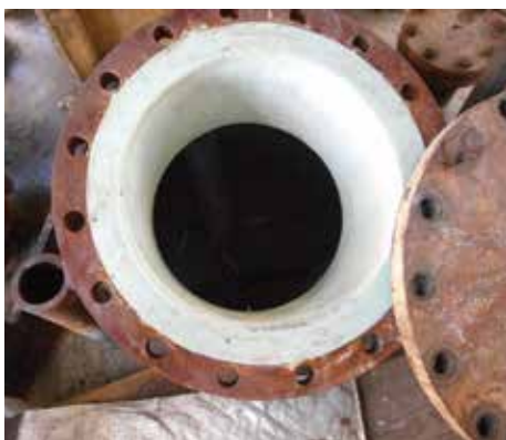
Above: Fig 4 and 5. Reactor inspected after 6 months in service
